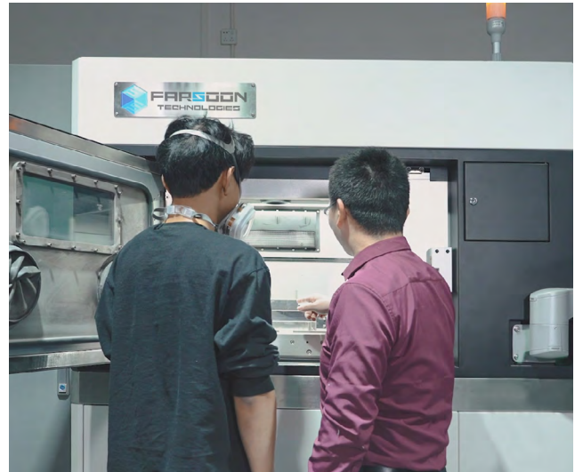
Figure 2: (Top) Farsoon FS273M dual-laser metal system installed in Borton Precision facility.
