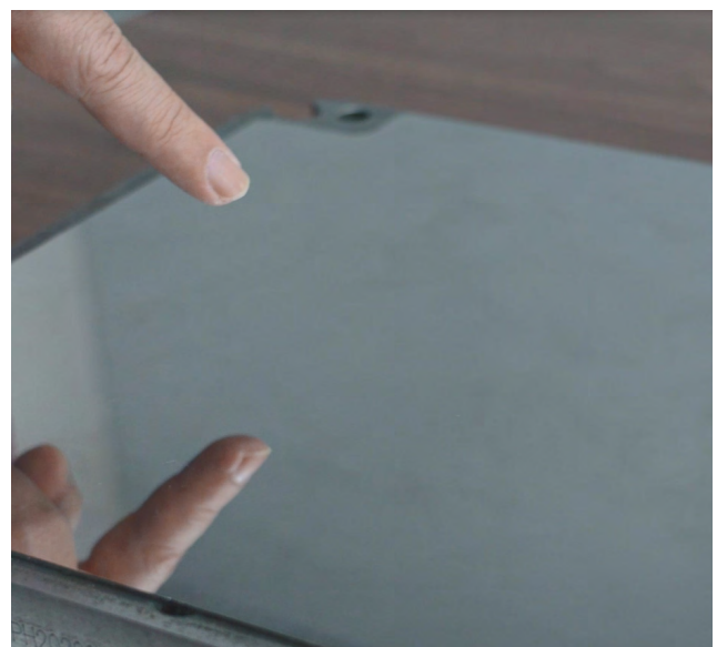
Figure 5: Grade A1 finish on a full FS273M base plate sized surface. Image Courtesy: Borton Precision
