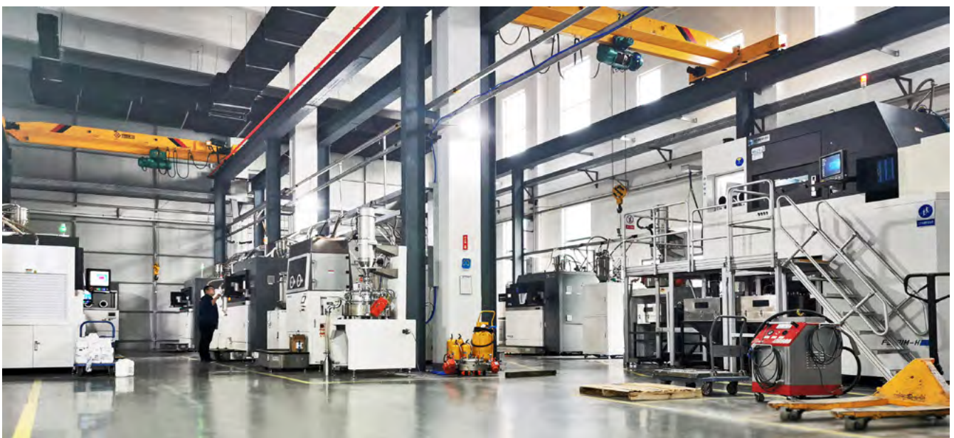
Figure 1: Falcontech Super AM Factory with currently 20 Farsoon metal 3D printing system.
